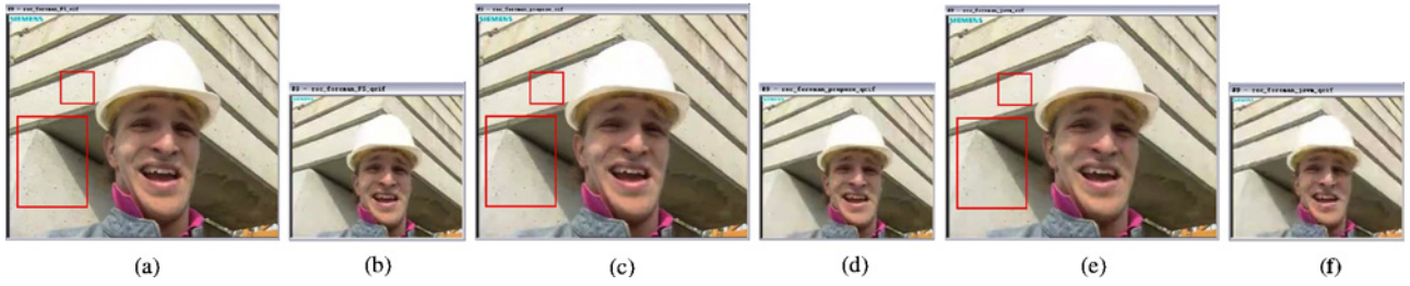
Fig. 15. Visual quality comparison among the proposed, JSVM and FS bit allocation schemes encoded by two spatial layers (QCIF–CIF), where the ninth frame of the Foreman sequence is shown. (a) FS, CIF. (b) FS, QCIF. (c) Proposed, CIF. (d) Proposed, QCIF. (e) JSVM, CIF. (f) JSVM, QCIF.
